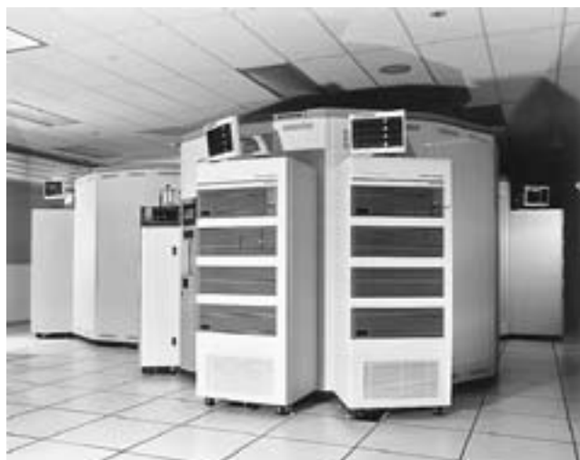
A NASA automated tape library. These facilities can store trillions of bytes of data. (NASA PHOTO)
